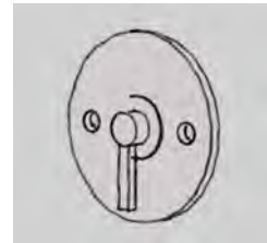
*Flue Damper Control Lever
