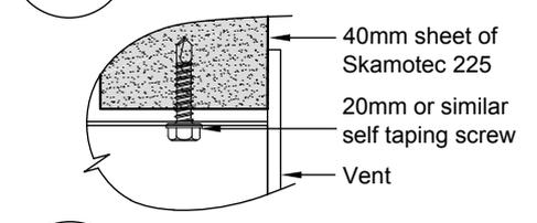
**C VENT FIXING DETAIL**
