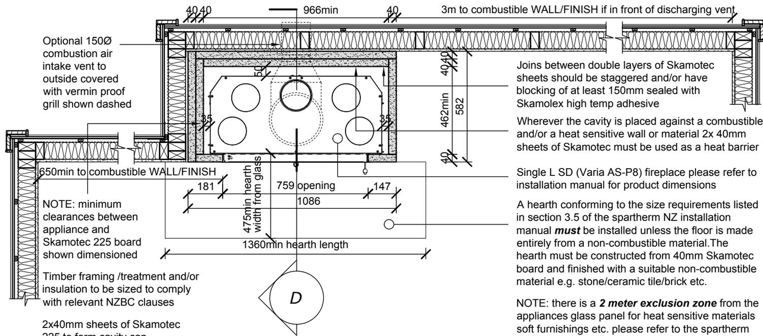
Joins between double layers of Skamotec sheets should be staggered and/or have blocking of at least 150mm sealed with Skamolex high temp adhesive
